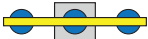
Center vacuum pad (1/3 capacity) used for short, narrow plates. Outer pads provided with shut-off valves.
