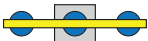
Center vacuum pad (1/3 capacity) used for short, narrow plates. Outer pads provided with shut-off valves.
