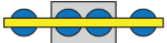
Center vacuum pads (1/2 capacity) used for short, narrow plates. Outer pads provided with shut-off valves.
