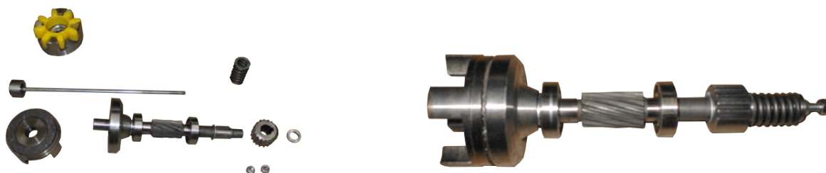
Diagram 6-19. Sliding Clutch Disassembled (l) and Assembled (r).
